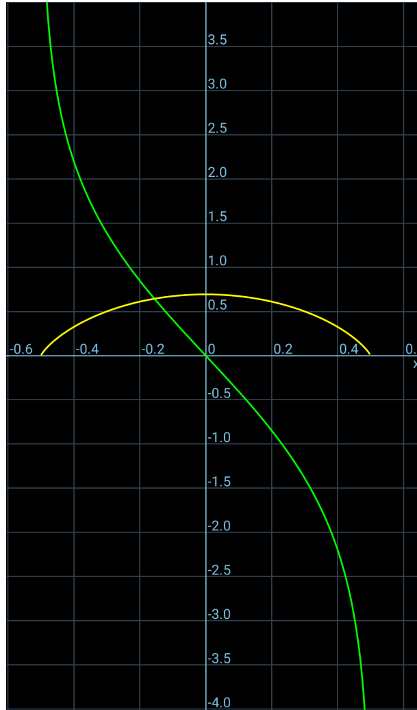
Figure 3.3: Entropy increment \Delta S_i (yellow) together with its derivative (green) according to 3.22
